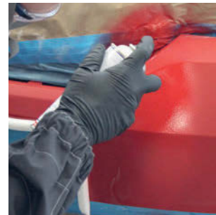
Apply Basecoat in 2-3 spray passes. Dry by air.
