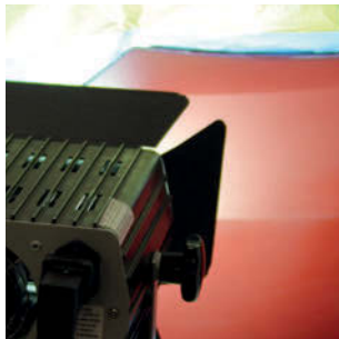
Dry UV-Filler for 4 minutes by using a UV-A Lamp with a wave length of 320-400 nm.
