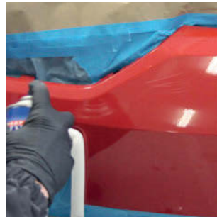
Clean surface generously with Silicone Remover.
