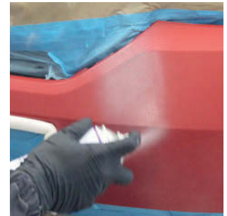
Shake UV Primer Filler for approx. 2 min and apply 1-2 spray passes (40-50 µm). Allow 1 min flash-off time.
